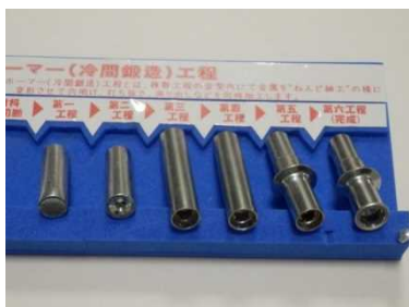
Cold-forged items after each process
