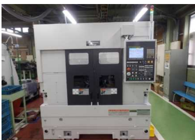
High precision NC equipment (parallel two-axis CNC lathe)
