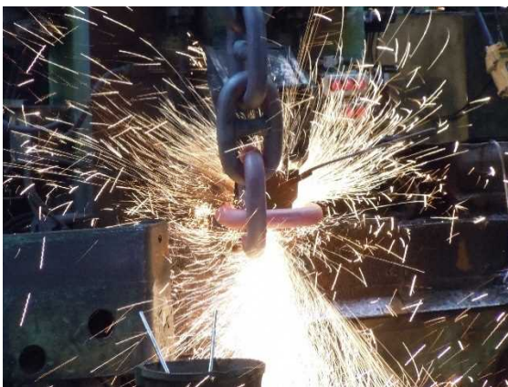
Sparks from flash butt welding
